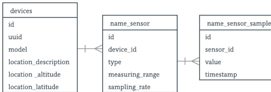
**Figure 1.** Basic data structure of the extended architecture of InCense.
