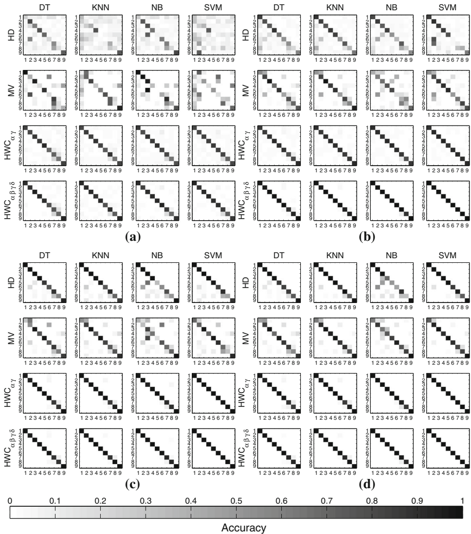
Fig. 4 Confusion matrices obtained from the experimental evaluation of each DF MARC modality (HD, MV, HWC \alpha\gamma , and HWC \alpha\beta\gamma\delta ) and machine learning paradigm (DT, KNN, NB, and SVM). Diverse feature vector lengths are considered; (a) 1, (b) 5, (c) 10, and (d) 20 features). Confusion matrix legend (activities): 1 walking, 2 running, 3 cycling, 4 sitting, 5 standing, 6 lying down, 7 stretching, 8 strength-training, 9 climbing stairs
